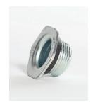
The metal plug VGII has an electro zinc chromate finish, rounded bottoms, and wide shoulders with concentric sealing beads to help lock gaskets securely into place. Known for it's distinctive flathead surface, the metal plug has no crossbar or dome features. This fitting is available in Zinc Plated or Buff Epoxy with White EDPM, Black Buna, or Poly Irradiated Gaskets. A Red Phenolic option is also available.
